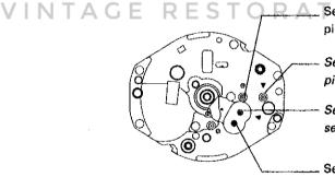
Set the small second wheel and pinion of Cal. 7N08A here.
