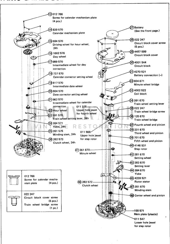
47) Disassembling procedures Figs.: Reassembling procedures Figs.: Lubricating: Types of oil Oil quantity Moebius A ○ Normal quantity ∞ SEIKO Watch Oil S-6 Silicone oil 500,000 c.s. Please see the remarks on the following pages. 1 Case Lack (6) Hour and minute (3) Case ring (7) Small hands 8) Dial 9 970 571 Date star 10 168 570 Hour correction wheel, 24h 11) 157 572 Hour wheel, 24h 12) 802 570 (5) Winding stem, 24h, with crown (4) Winding stem Date driving wheel with crown
