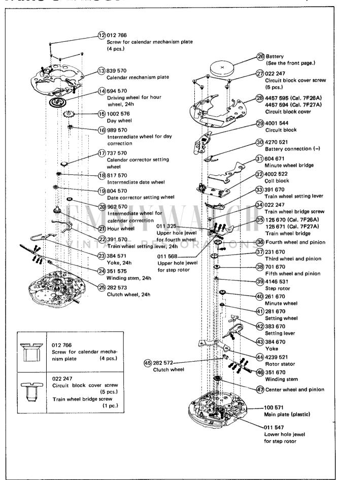
48) Disassembling procedures Figs.: (1) Reassembling procedures Figs.: Oil quantity Lubricating: Types of oil Moebius A ∞ SEIKO Watch Oil S-6 Silicone oil 500,000 c.s. Please see the remarks on the following pages. 1 Case back 2) Case back gasket 6 Hour and minute hands 3 Case ring 7) Small hands 8 Dial 9)970 571 Date star 10 168 570 Hour correction wheel, 24h 11) 157 572 Hour wheel, 24h 12)802 570 Date driving wheel (4) Winding stem (5) Winding stem, 24h, with crown with crown
