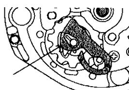
Insert a tip of tweezers or the like into the part indicated by the arrow in the illustration, and remove the moon phase finger.
