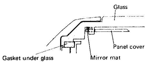
The panel cover is fixed with a mirror mat which is fixed to the glass.
