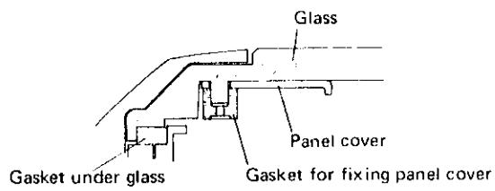
The panel cover is fixed with a gasket for fixing panel cover to the glass.
