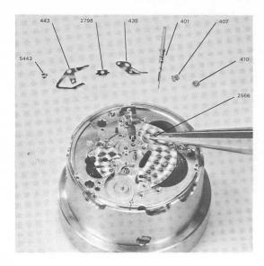
8.1.11 Take out the screw (5443). Remove in order the yoke 435, the setting lever 443, the sliding pinion 407, the winding pinion 410, the date-corrector maintaining plate 2798, the date-corrector 2566 and the winding stem 401 or 404.
